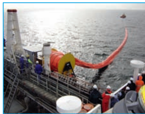
EMSA vessels deploying sweeping arms (left) and offshore boom (right)
