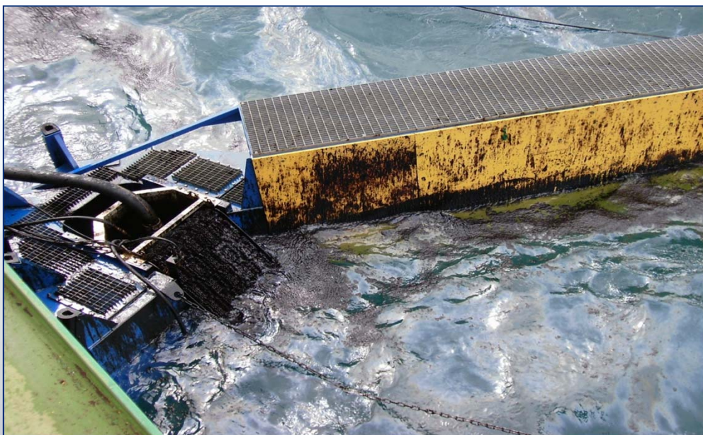
Rigid Sweeping Arm with integrated brush skimmer
