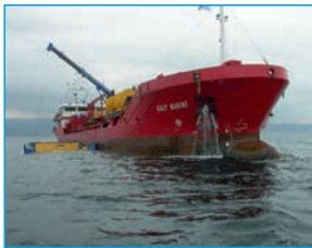
EMSA vessels deploying sweeping arms (left) and offshore boom (right)
