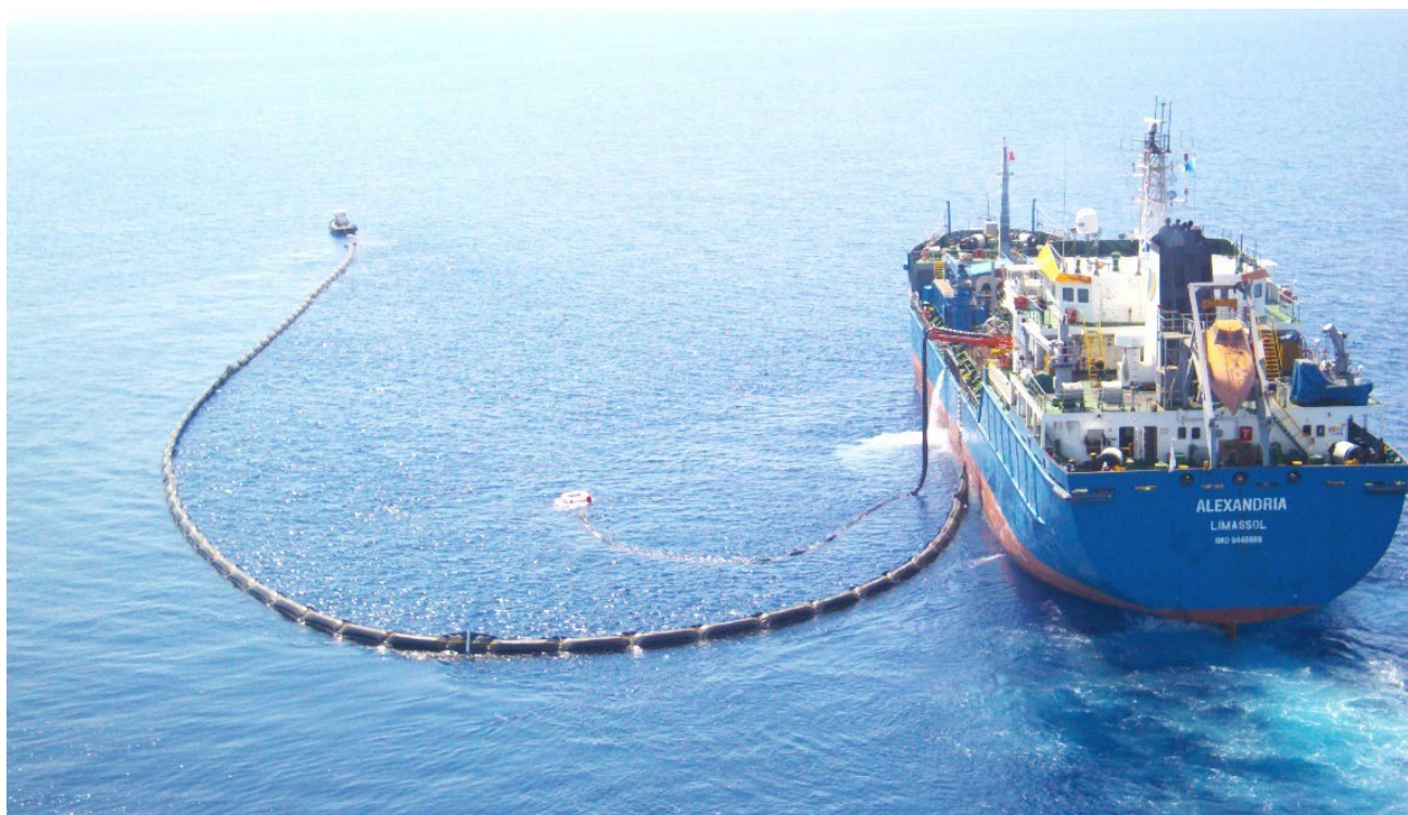
Fig. 2. Quarterly drill on board Aalexandria. Deployment of the boom and high capacity skimmer.
