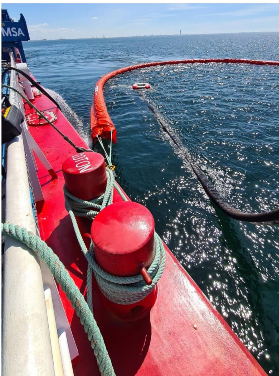
Fig. 2. Quarterly drill on board Norden . High capacity skimmer and boom in J formation.
