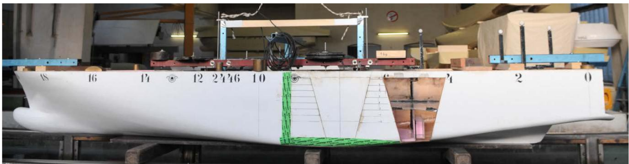
Figure 26 - Hull breach according to ( 8 ) and ( 9 ), SHIP 1, physical model test, case R7_P6-7.4.0
