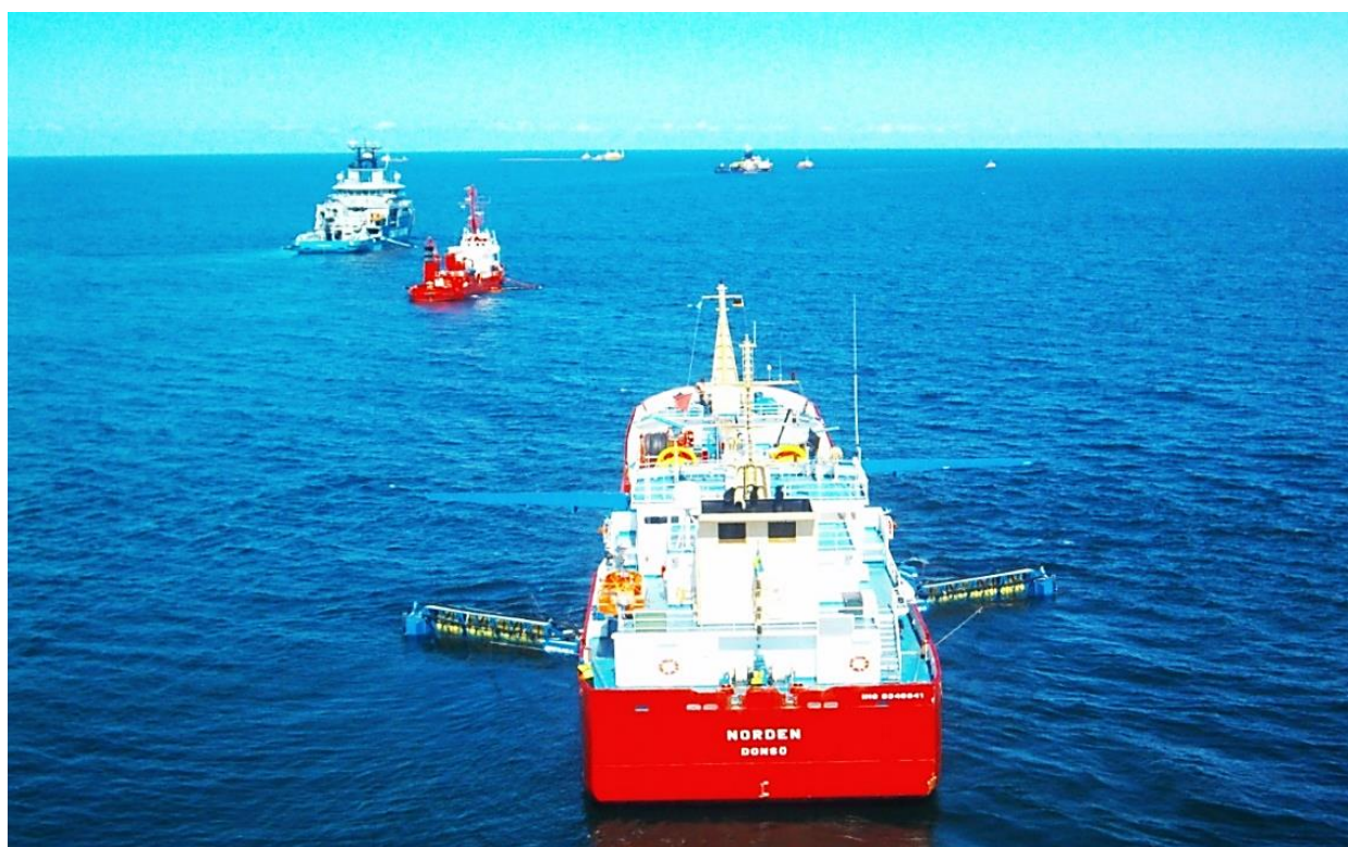
Figure 10: BALEX DELTA 2022 exercise - Oil pollution response. Strike team DELTA composed of KBV 003 Amphitrite (strike team leader), Norden and Kiel vessel of the German National Fire brigade.
