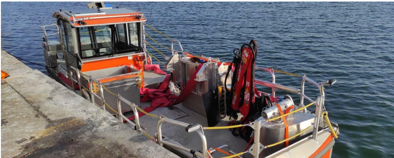
Figure 8: ECT V-sweep system in EAS Black Sea
