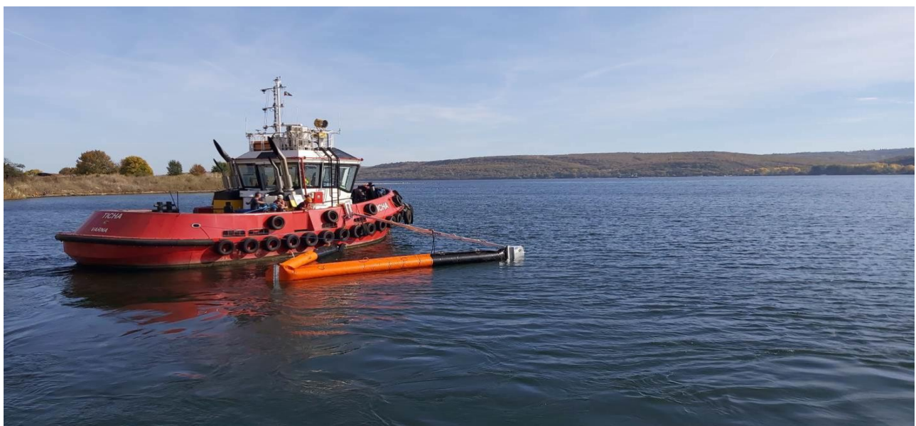
Figure 8: ECT V-sweep system in EAS Black Sea
