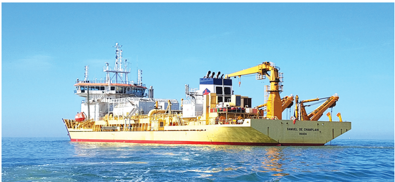
Image A5.3 The SamuelLNG vessel, Samuel de Champlain: first European dual-fuel converted dredger
