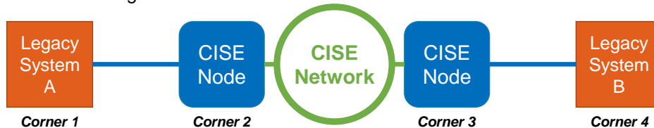
Figure 13. Four corners in the communication protocol.
