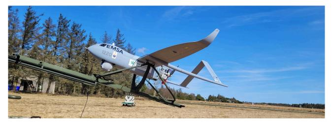
The RPAS service is delivered by EMSA through the contractor Nordic Unmanned AS operating an Aerosonde RPAS over a four-month period. The RPAS uses a catapult for take-off and is recovered with a net, has an endurance of 10 hours and a radio range of 140 km which can be extended based on ground relay stations. It is equipped with both an optical and infrared camera, as well as an AIS receiver.
