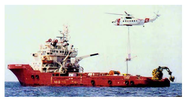
Figure 17. A Sikorski 61N helicopter reloading a RESPONSE 3000 dispersant spray bucket from dispersant stored onboard a support vessel
