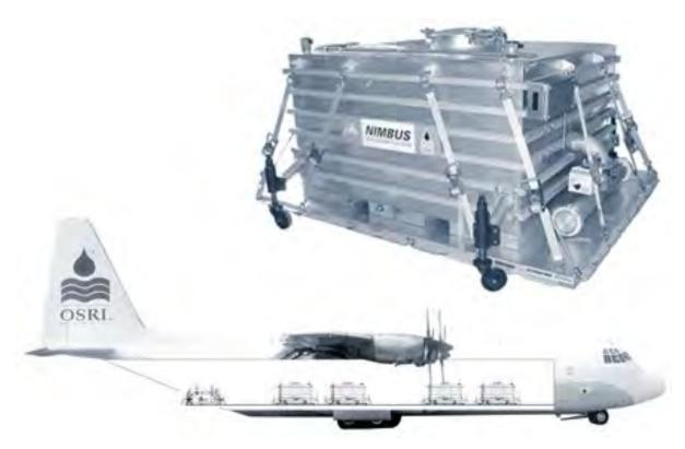
Figure 16. Lockheed L-382 Hercules aircraft with Nimbus spray system
