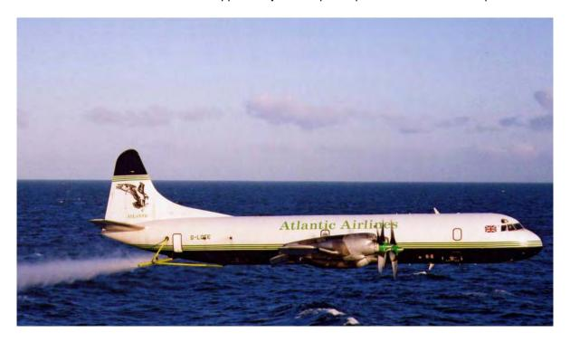
Figure 14. Lockheed Electra aircraft spraying dispersant
