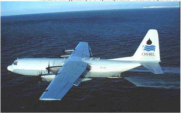
Figure 15. Lockheed L-382 Hercules aircraft with Airborne Dispersant Delivery System (ADDS Pack)
