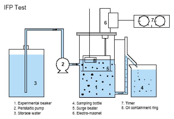
Figure 24. The IFP test apparatus
