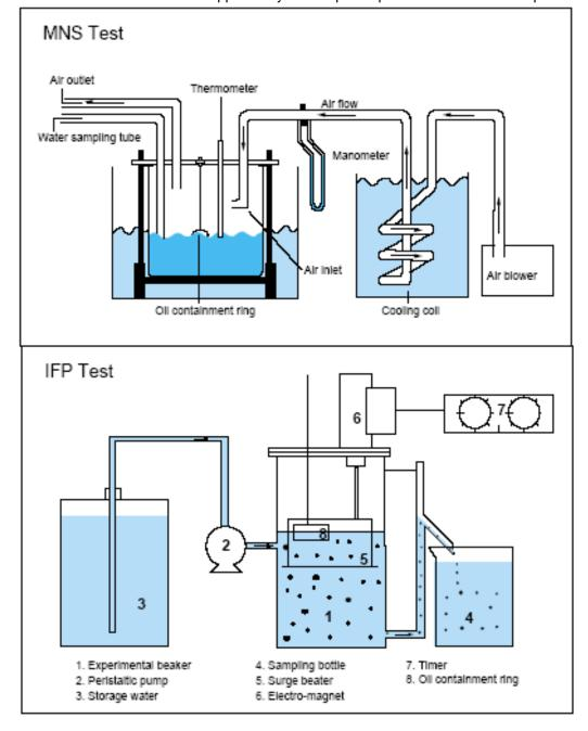
Figure 6. The MNS and IFP dispersant test methods
