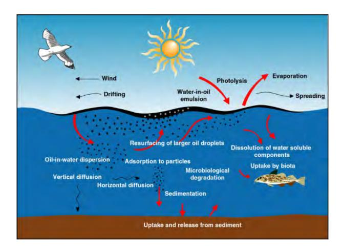
Figure 3. Weathering processes of spilled oils
