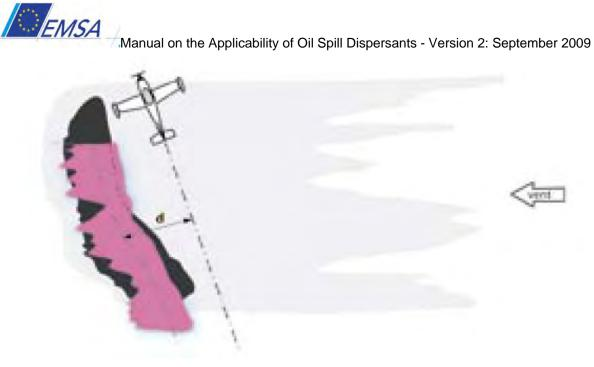
Spraying dispersant from a fixed-wing aircraft at an angle to the prevailing wind Figure 19.
