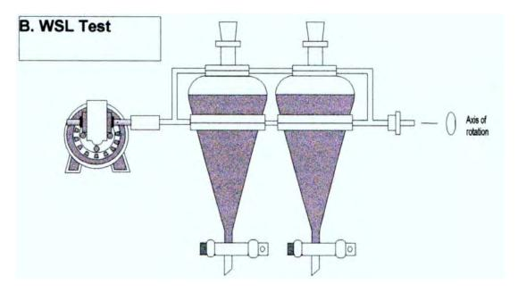
Figure 23. The WSL test apparatus
