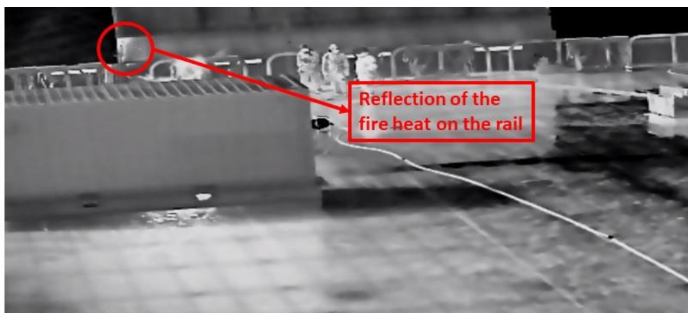
Figure 23. Picture of fire detection for test 2 – Thermal imaging camera.
