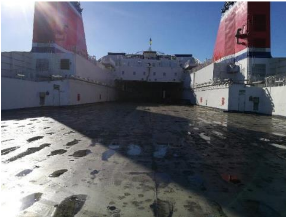
Figure 11. The aft of the test vessel showing the weather deck of deck 7 and the aft opening of the open ro-ro space.
