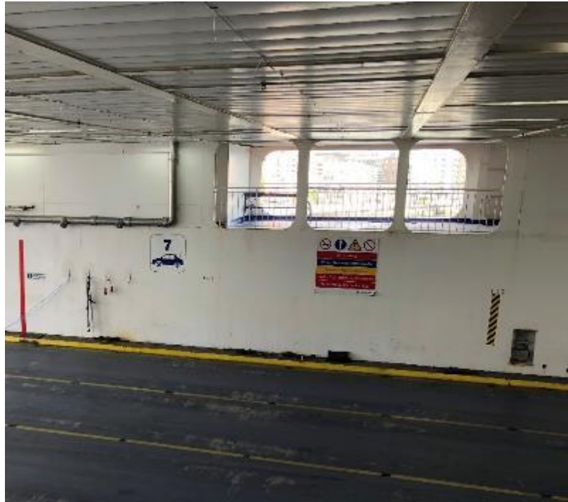
Figure 13. Side openings of the open ro-ro space.
