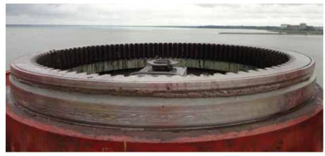
Failure of deck crane slewing ring bearing, MV SEAPACE, 13/8/2014
