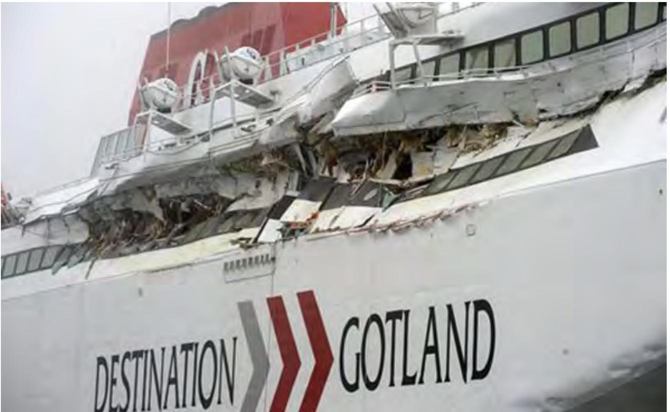
Substantial damage to the ferry *Gotlandia II*, after the collision with the *Gotland* at the port of Nynashamn (Sweden) during July 2009.
