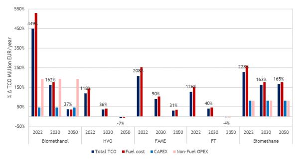
Figure 30. Annual difference in TCO of alternative fuelled bulk ships (35,000-59,999 dwt) with increased bunkering
