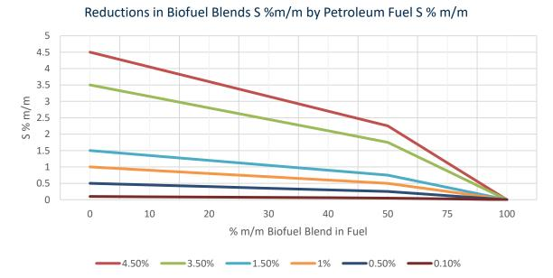
Figure 36. Reductions in % S in fuel with different Biofuel Blends
