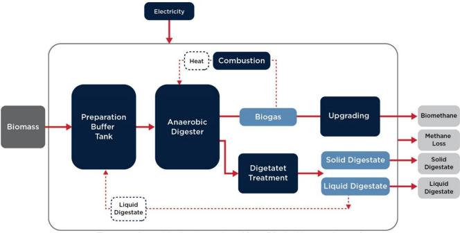
Figure 16. Anaerobic digestion, adapted from (Moghaddam, et al., 2019)
