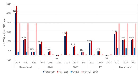
Figure 33. Annual TCO of alternative-fuelled containerships (14,500-20,000 TEU) with increased fuel storage
