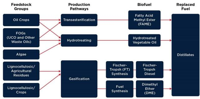
Figure 2. Production Pathways for Biodiesels
