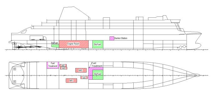
Figure 41. General Arrangement of the RoPax Vessel
