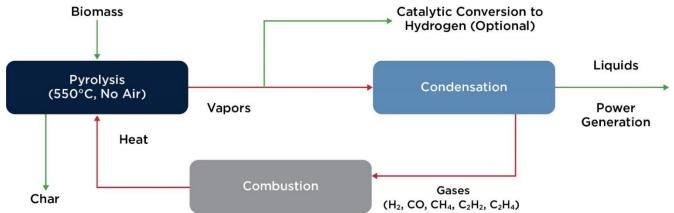
Figure 11. Biomass liquefaction via pyrolysis, adapted from (Zafar 2021)
