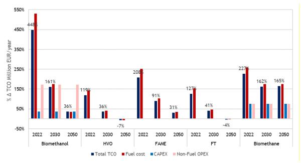
Figure 32. Annual TCO of alternative-fuelled containerships (14,500–20,000 TEU) with increased bunkering The following significant outcomes concerning the difference in yearly TCO of alternative fuelled containerships is outlined:
