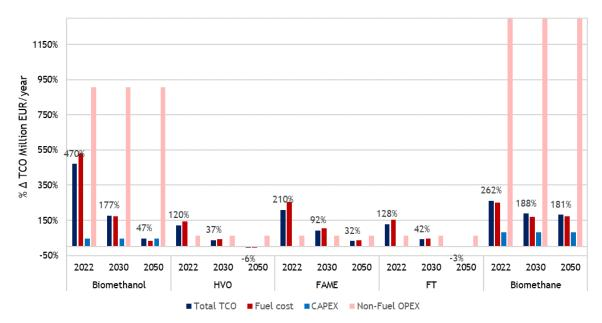
Figure 31. Annual TCO of alternative-fuelled bulk ships (35,000-59,999 dwt) with increased fuel storage
