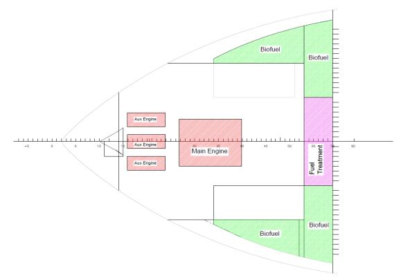
Figure 42. General Arrangements of the VLCC vessel
