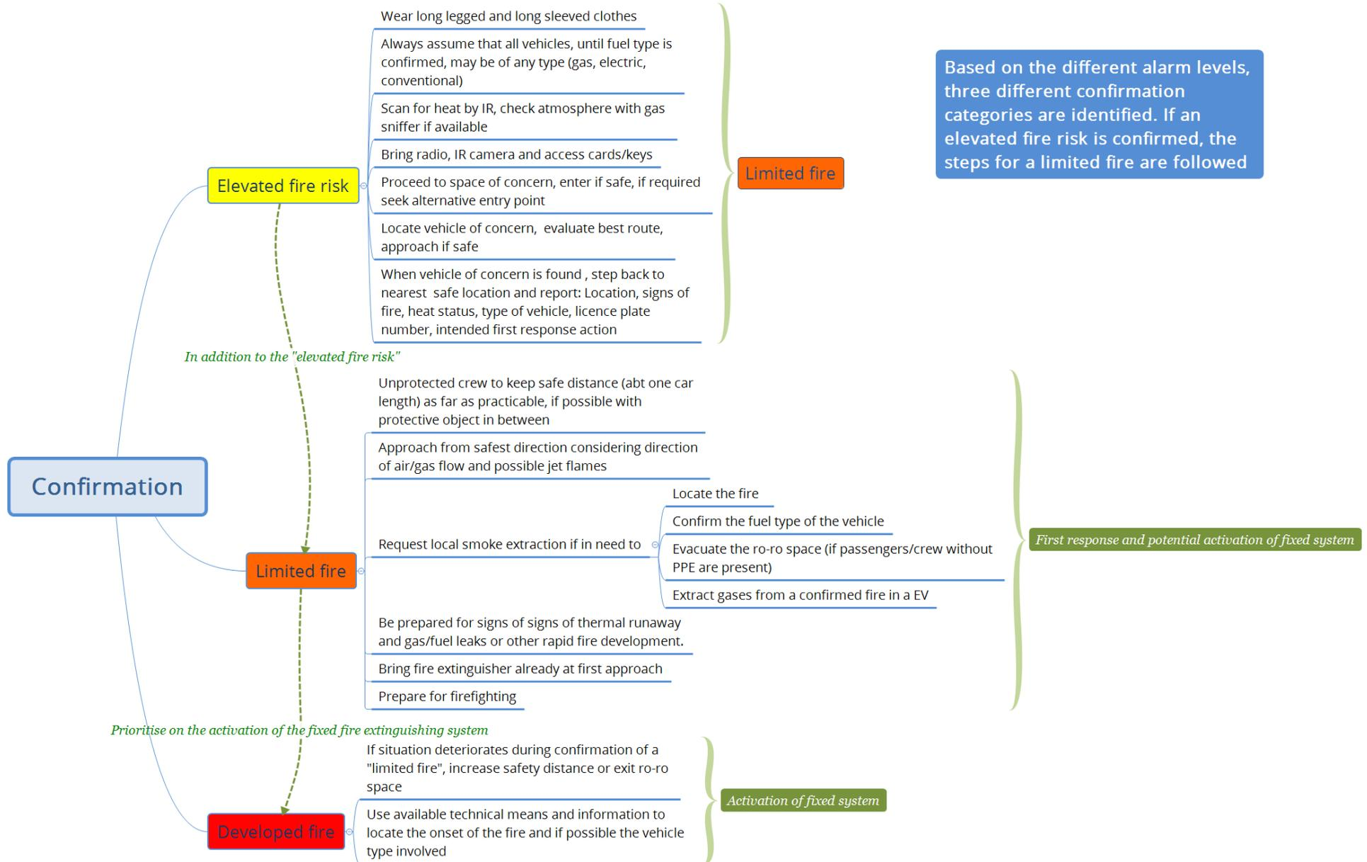
The intention of elementary first response is that of a possible fast reaction to a minor/initiating event by an unprotected crew member
