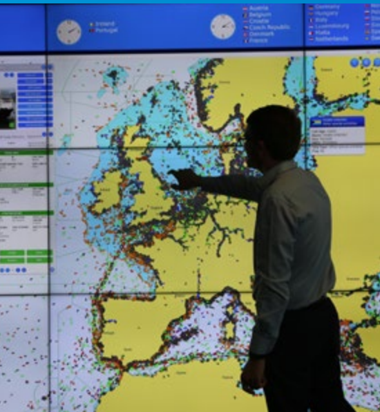
Heat map generated with the EMSA maritime analytics tool, displaying drifting events over a 24-hour period as detected using Automated Behaviour Monitoring algorithms running globally.
