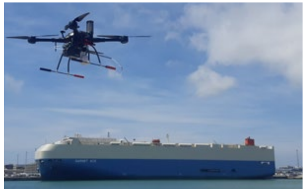
RPAS equipped with gas sensors can take measurements of air emissions from ships
