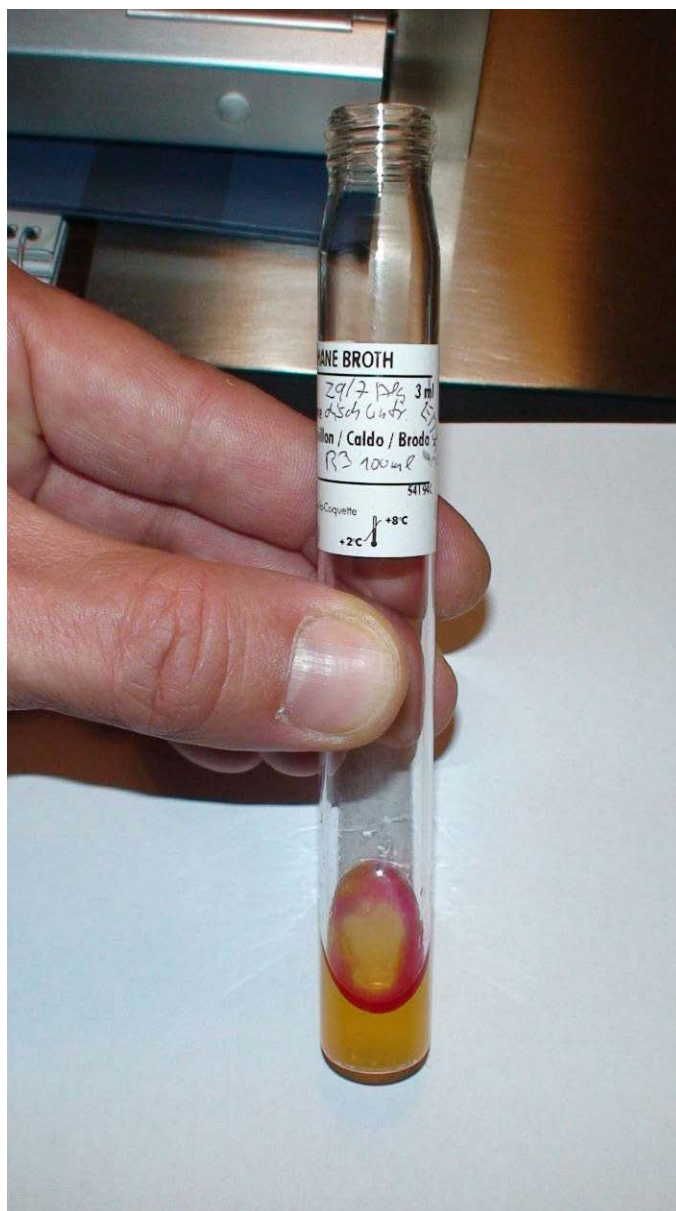
Figure 27 E. coli samples, second incubation step with Tryptophane broth in glass tube after addition of two drops of Kovac solution. The colour change on the surface to red confirms the presence of E. coli .
