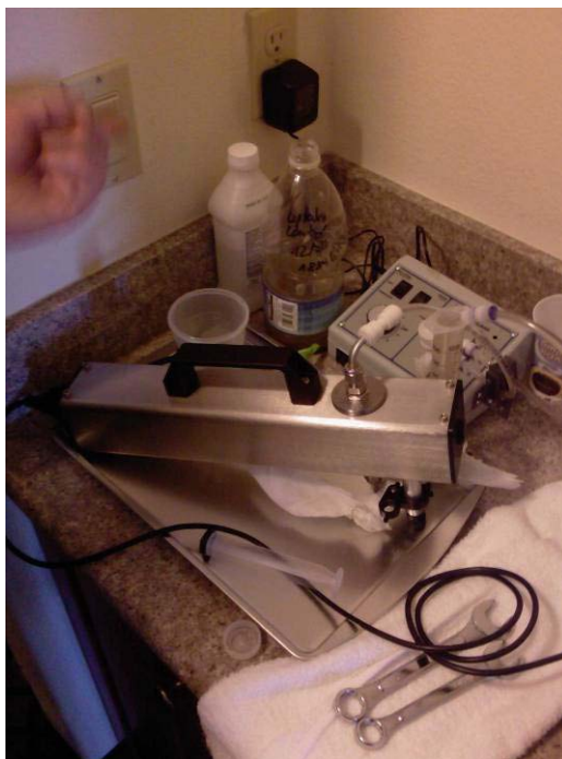
Figure 50 The hand-held flow camera of Fluid Imaging Technologies, Inc, USA.
