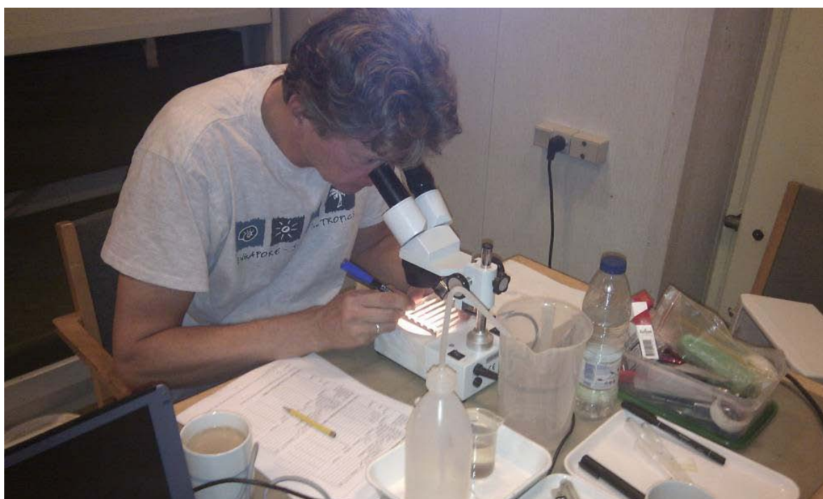
Figure 18 Onboard counting of organisms greater and equal to 50 micrometres in minimum dimension using a stereomicroscope.
