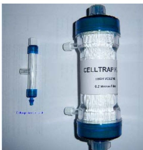
Figure 54 The Cell Trap of Harvey-Coleman Ltd, UK (Photo modified from www.harvey-coleman.com ).
