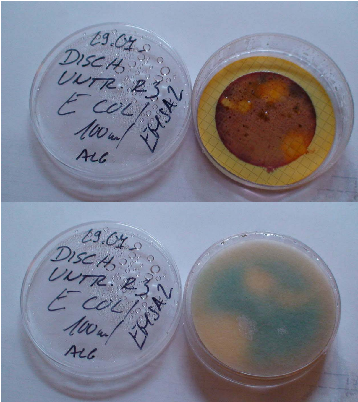
Figure 25 E. coli test plates after incubation. Transparent E. coli "suspects" (top) and yellow halos visible from underneath the Petri dish (bottom).
