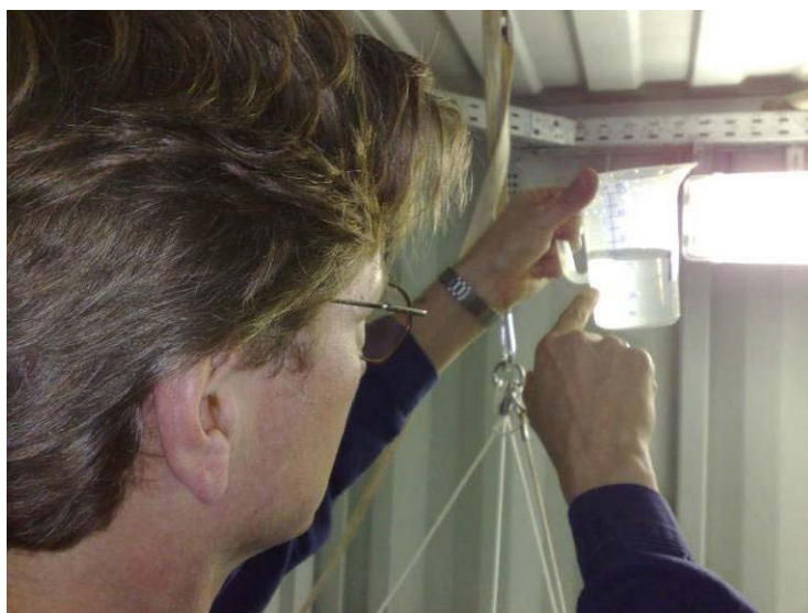
Figure 51 Inspection of an unconcentrated ballast water sample at the sampling point.
