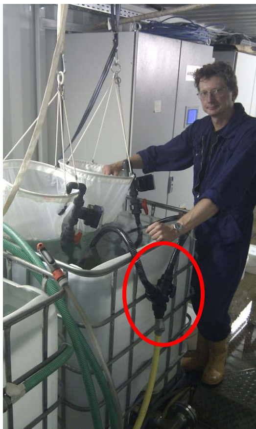
Figure 11 The flow splitter arrangement (red circle).
