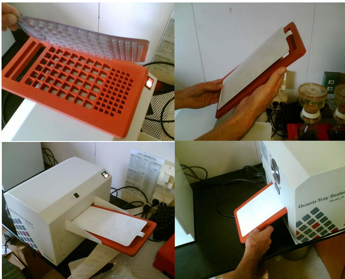
Figure 58 Sealing of IDEXX incubation plates.
