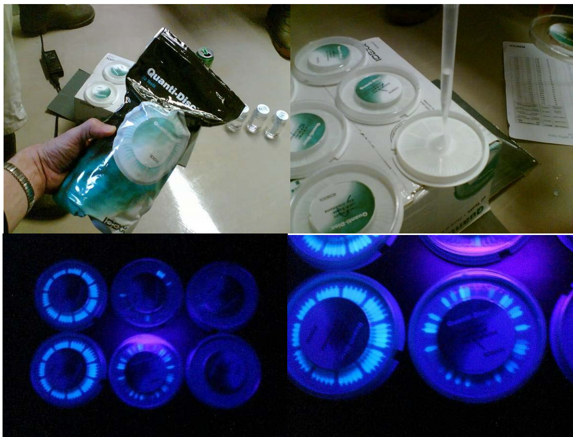
Figure 59 IDEXX Quanti-Disc trial for total bacteria. Test with three dilutions (bottom left, left disc undiluted, middle 10 ml and right 1 ml bacteria solution filled to 100 ml with distilled water). Bottom right is a close up of the left image.
