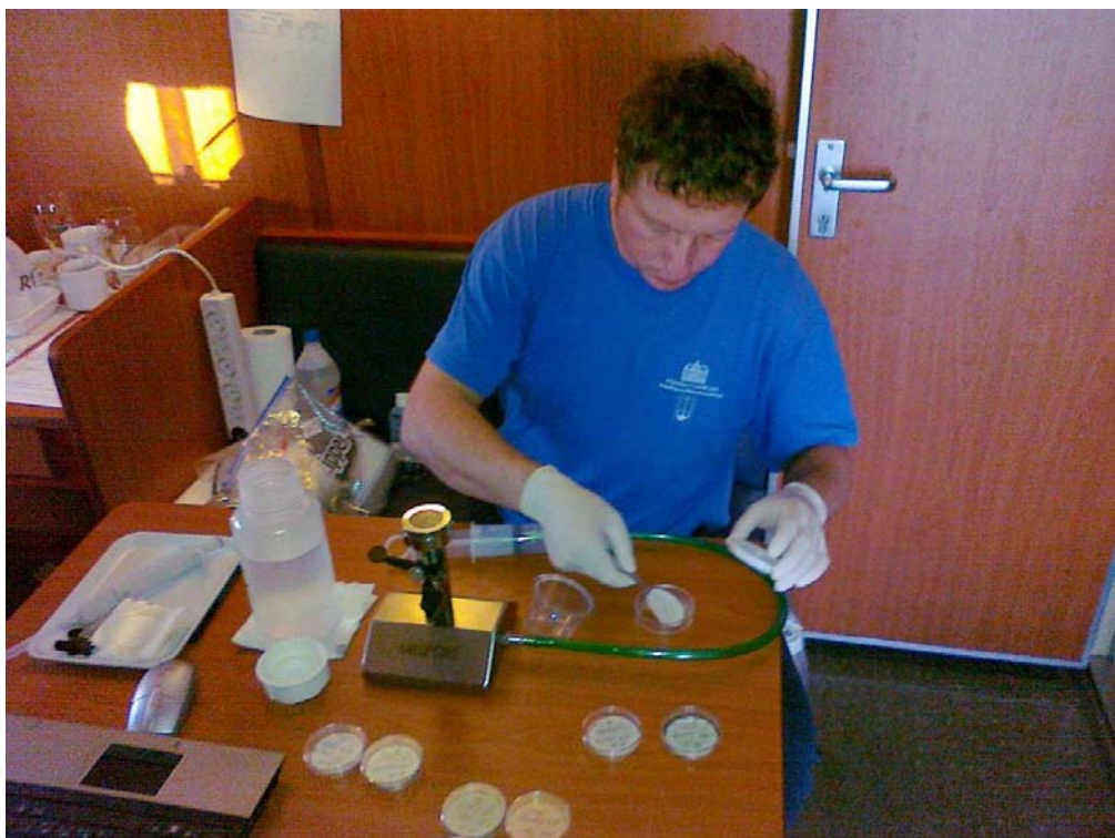
Figure 22 Transfer of filter plates from Millipore stand to Petri dish.
