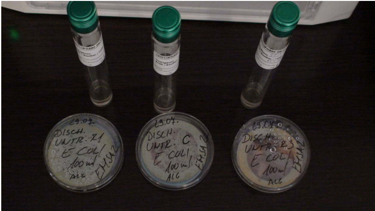
Figure 26 E. coli test plates after incubation also showing glass test tubes with Tryptophane broth (second incubation step).
