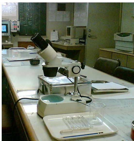
Figure 52 A stereo-microscope in use for on-board analysis of organisms greater than or equal to 50 micrometres in minimum dimension. A Bogorov counting chamber is shown on the white tray in the foreground.
