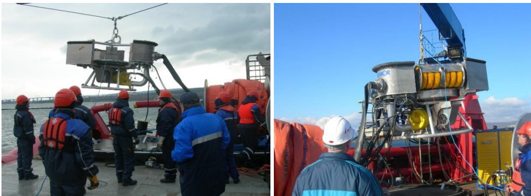
Weir Skimmer LWS 1300 Mk II with brush and weir modules
