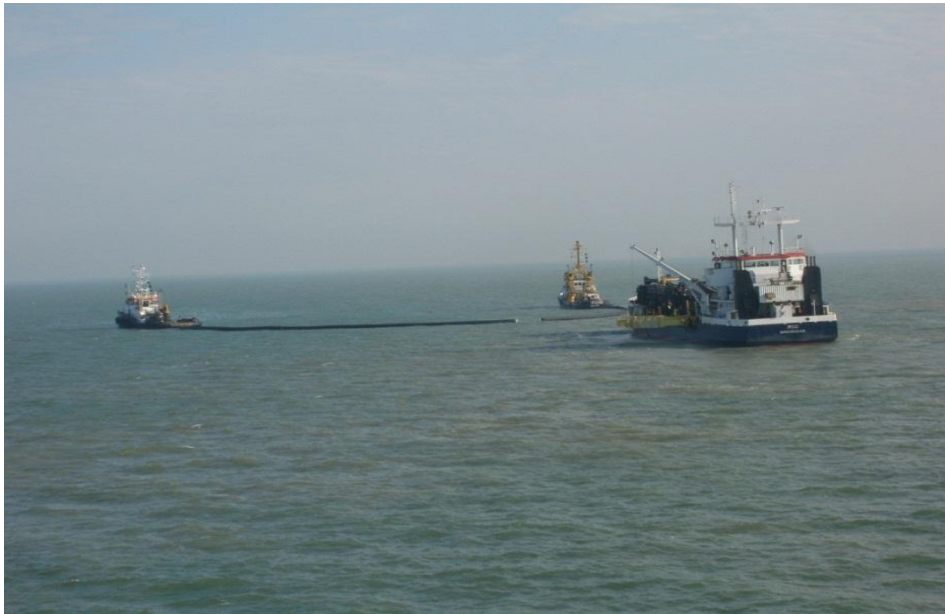
Picture 14: Dredger with deployed sweeping arms following open U formation
