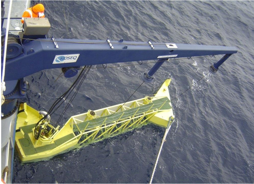
Picture 16: Salina Bay with the starboard sweeping arm deployed
