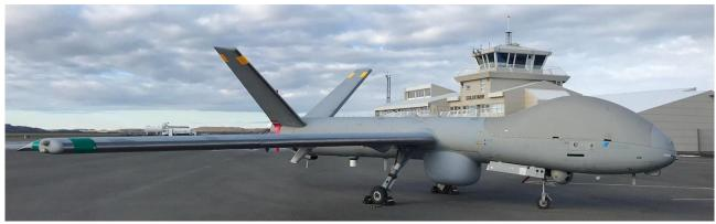
The particular RPAS in use is adapted to withstand the strong winds and icy conditions common to the North Atlantic Ocean. It has an endurance of over 12 hours and may perform maritime surveillance tasks in areas extending as far as 200nm from the shoreline. The operations are based at the Egilsstaðir airport in the east of the island. From there, they have the capability to cover more than half of the Icelandic Exclusive Economic Zone.
