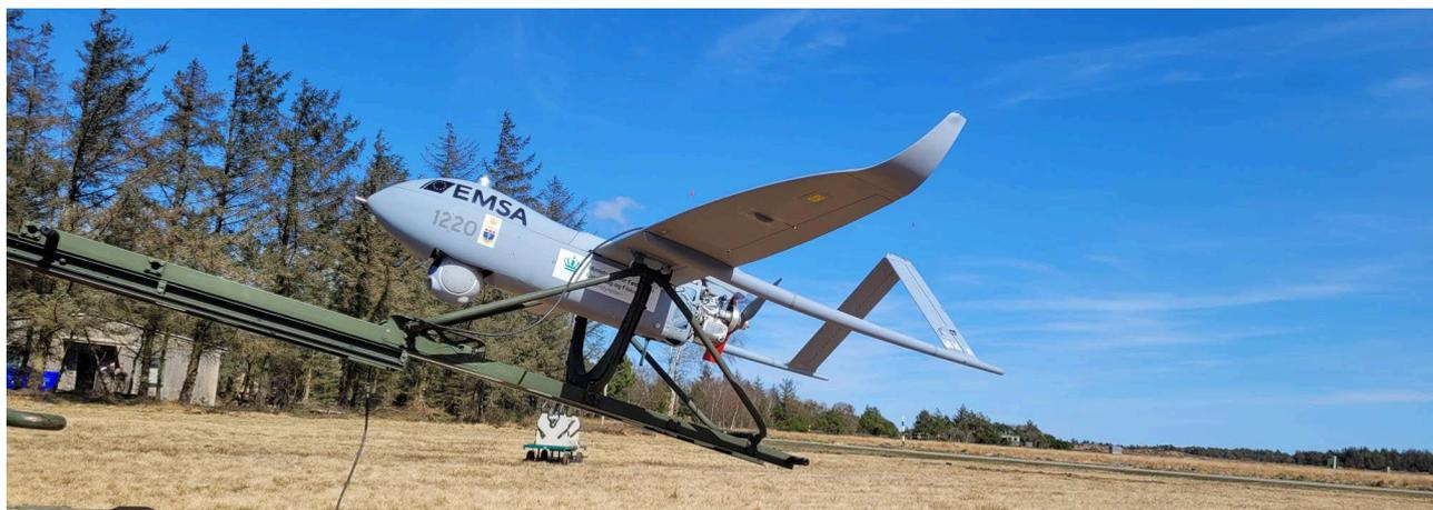
The RPAS service is delivered by EMSA through the contractor Nordic Unmanned AS operating an Aerosonde RPAS over a four-month period. The RPAS uses a catapult for take-off and is recovered with a net, has an endurance of 10 hours and a radio range of 140 km which can be extended based on ground relay stations. It is equipped with both an optical and infrared camera, as well as an AIS receiver.
