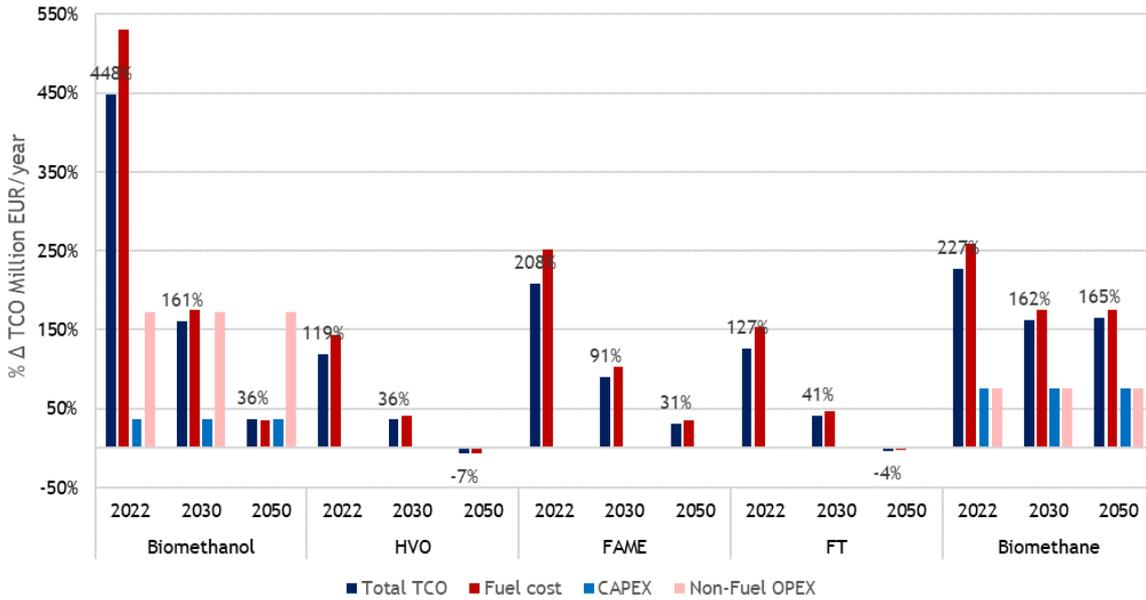
Figure 32. Annual TCO of alternative-fueled containerships (14,500–20,000 TEU) with increased bunkering. The following significant outcomes concerning the difference in yearly TCO of alternative fuelled containerships is outlined:
