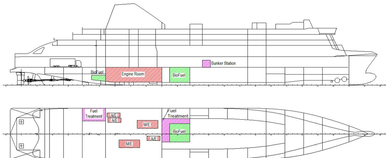
Figure 41. General Arrangement of the RoPax Vessel
