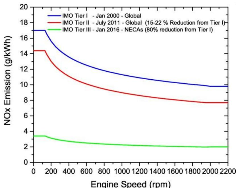
Figure 34. MARPOL 73/78 Annex VI Reg 13 - NOx emission limits with respect to engine speed
