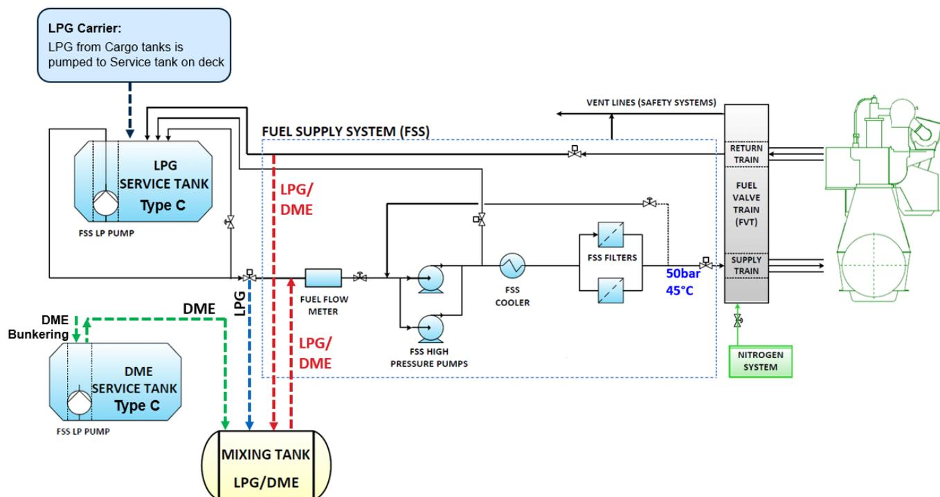
Figure 45: Schematic of the LPG/DME fuel supply system (for illustration purposes only).
