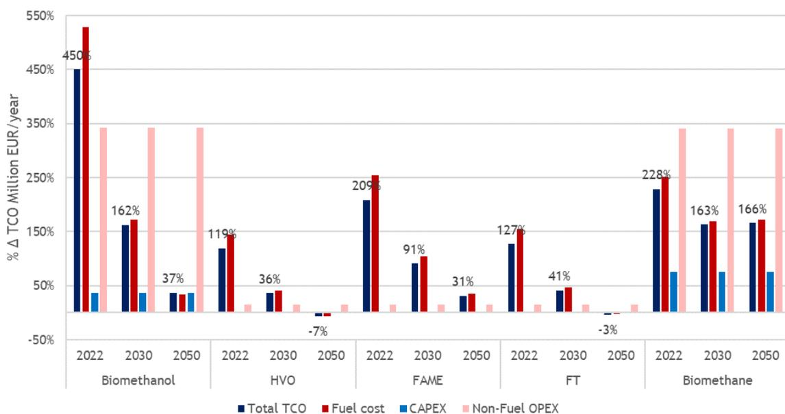
Figure 33. Annual TCO of alternative-fueled containerships (14,500–20,000 TEU) with increased fuel storage
