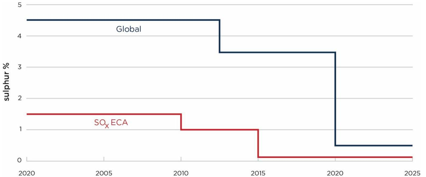
Figure 35. MARPOL 73/78 Annex VI Reg 14 – % Sulphur content in fuel limits
