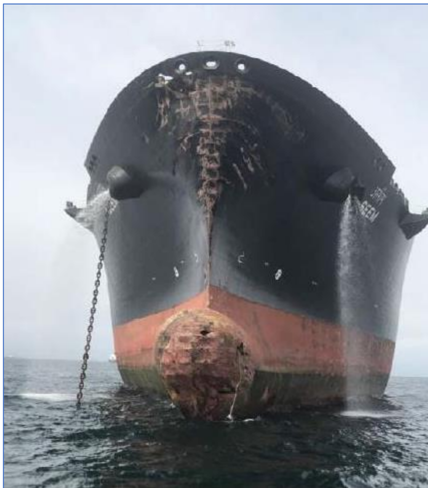
Figure 3 – Collision between LNG Carrier “Aseem” and VLCC “Shinyo Ocean” within the passage channel of the Fujairah Offshore Anchorage Area, UAE on 25/03/2019 – MSIU (Malta)
