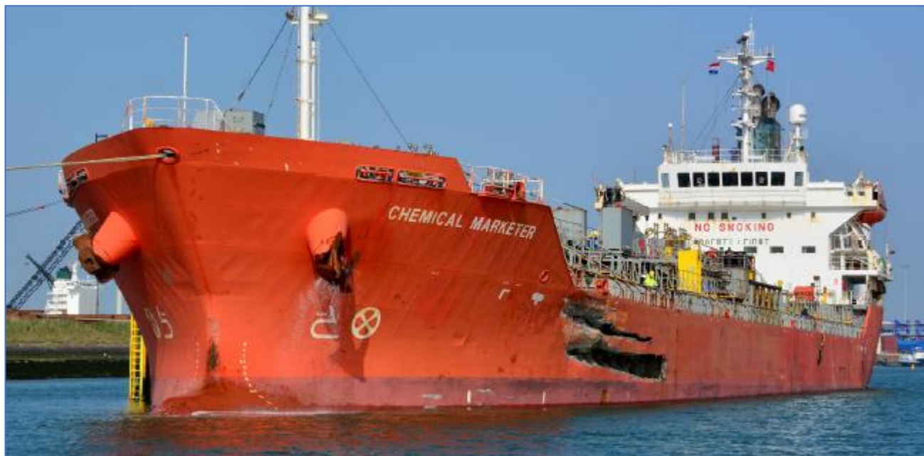
Figure 13 – Collision between the River cruise ship “Viking Idun” and the chemical tanker “Chemical Marketer” on the Western Scheldt on 01/04/2019 – DSB (the Netherlands)
