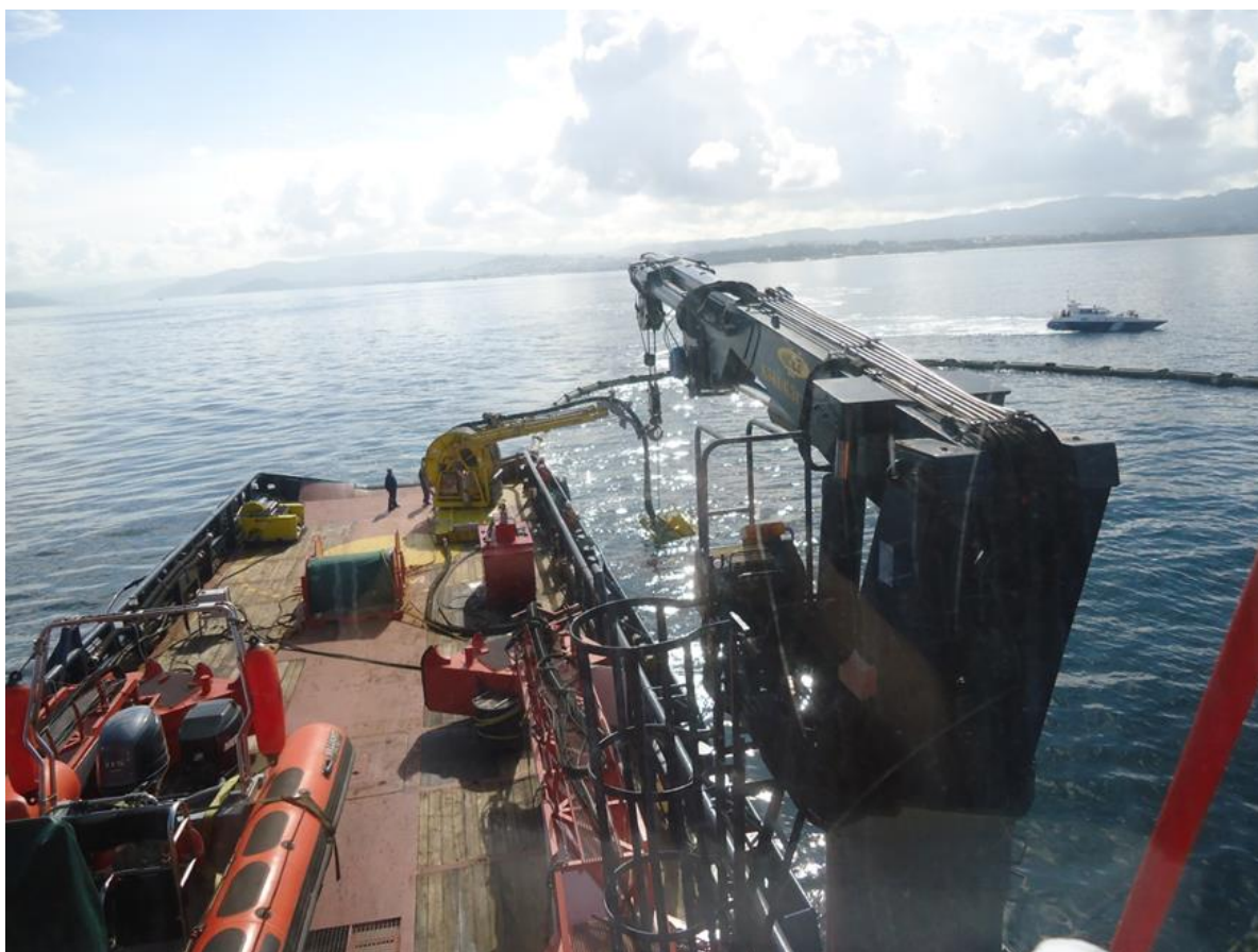
Ria de Vigo deploying the Transrec High Capacity Skimmer System during the SASEMAR-EMSA Atlantic 2013 Exercise
