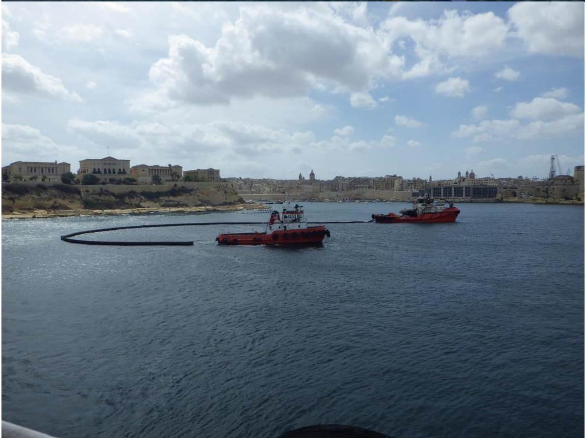
Exercise Maltex 2013. Tugs Spinola and Felicia towing the boom in "U" formation
