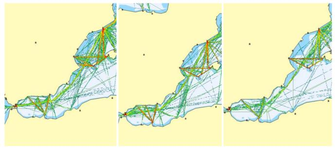
Figure 9: Passenger ship traffic density in January 2019 (left), in January 2020 (centre) and in January 2021 (right)
