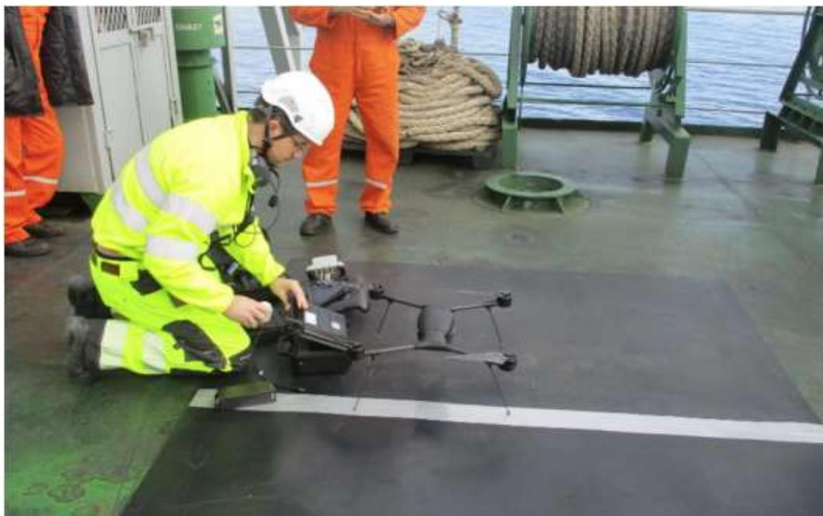
*Figure 22 - Pilot preparing the RPAS to take-off from an EMSA pollution response vessel.*
