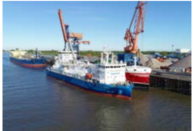
Image 16: NAUTICOR 7,500m 3 LNG bunker vessel MV Kairos.
