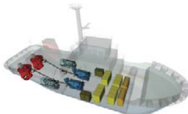
Figure 124: Battery powered tug design – hybrid tug system - IHI Power Systems Co., Ltd.
