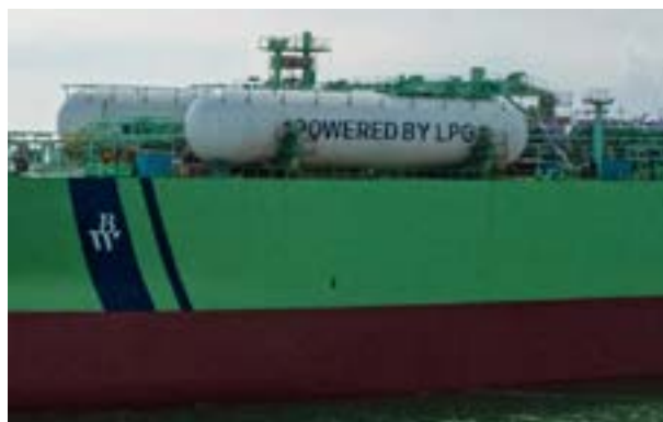
Image 22: BW MV Gemini, LPG fuel tanks.
