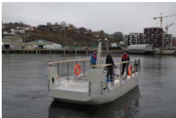
Image 12: The full-scale autonomous ferry prototype milliAmpere II.
