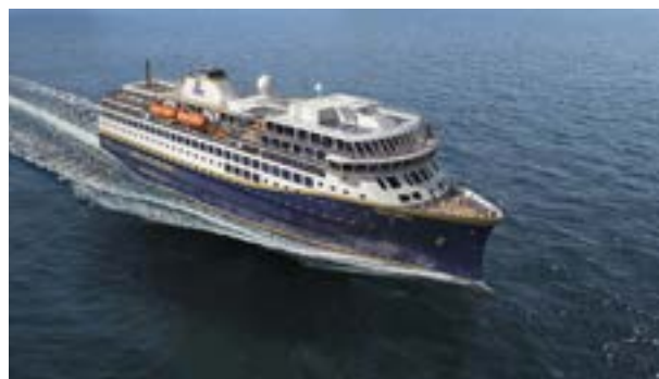
Figure 128: Project for a hydrogen fuelled, 3.2MW fuel cell powered passenger ship, currently being designed by Havyard Design for the shipowner.
