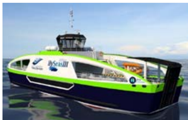
Figure 129: HySeas III – the third development stage of EU funded project to deliver a ferry powered by hydrogen fuel cells.
