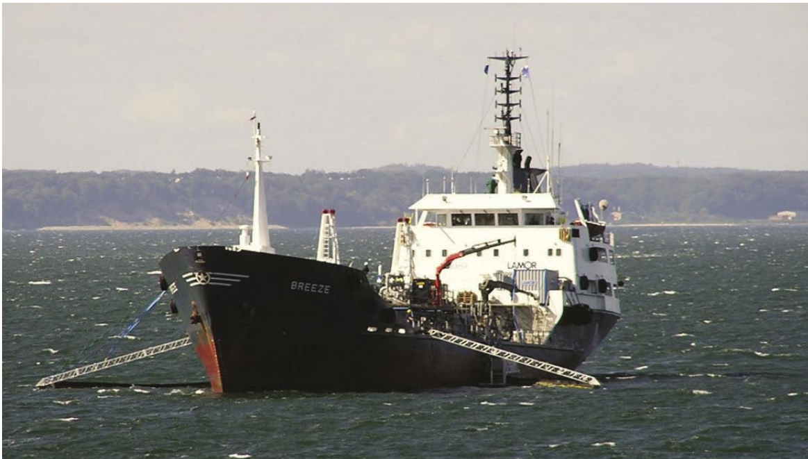
EMSA contracted vessel Breeze with sweeping arms deployed during the HELCOM BALEX Exercise 2006.
