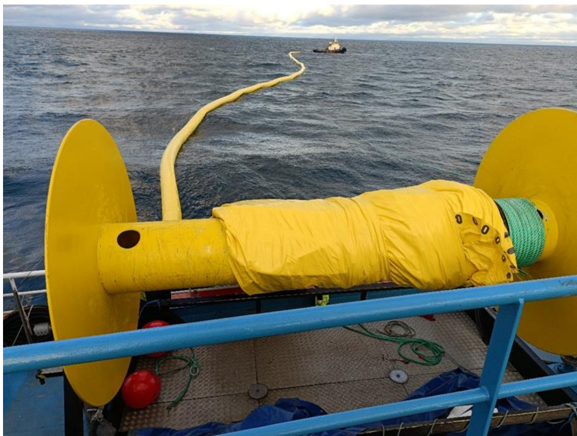
Figure 1. 4 th Quarterly drill on board Norden . Oil boom deployment.
