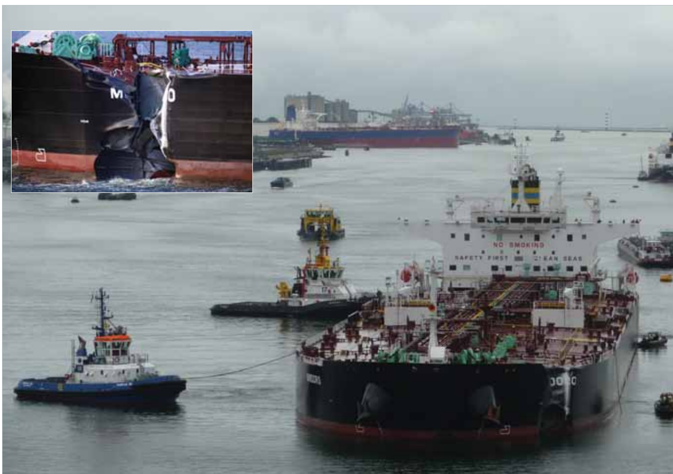
The Mindoro suffered a large gash to the port side of the hull (see photo, inset).
