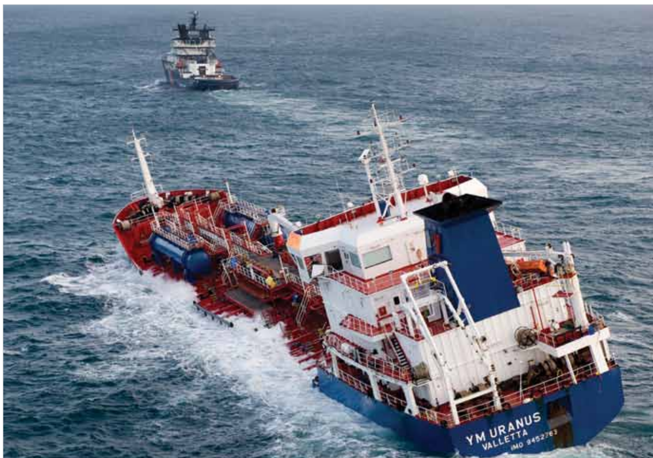
The YM Uranus accident illustrated how a double hull design helped to prevent a potentially serious marine pollution accident.
