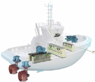
Figure 143: Battery powered tug boat design of integrated power systems by Kongsberg Maritime AS.
