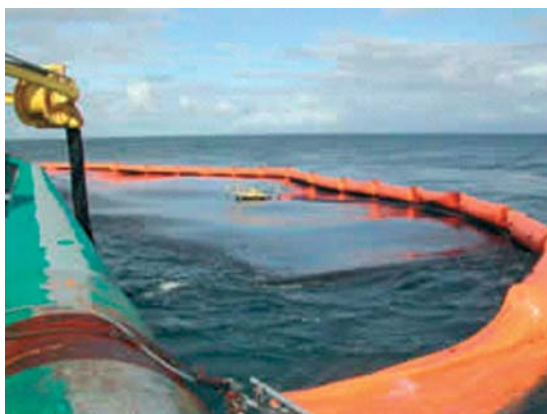
Vessel with Boom and Skimmer System Deployed
