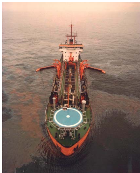
Vessel with Sweeping Arm System Deployed
