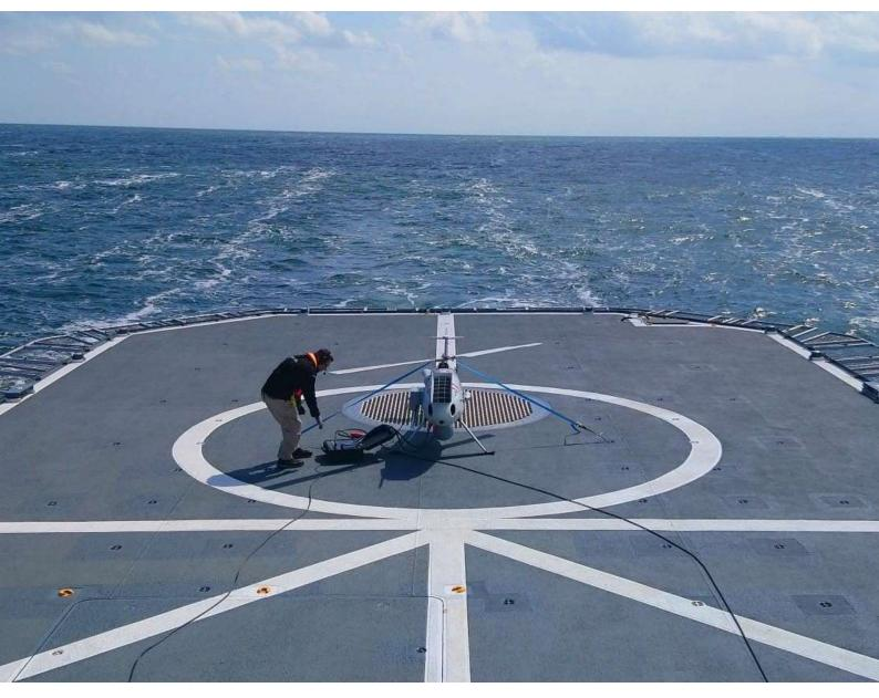
Figure 19 - RPAS on board a German Police vessel for emissions monitoring 2024
