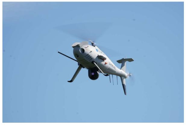
Figure 33- RPAS equipped with an emissions monitoring sensor
