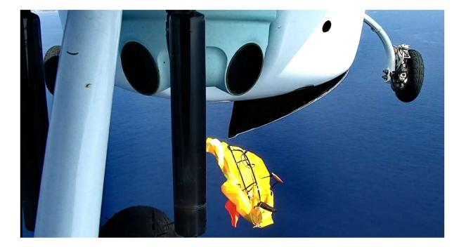
Figure 4 - RPAS dropping a life raft during a SAR exercise, Italy, 2023
