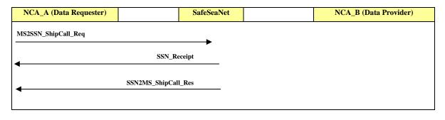
Flow of XML messages when the 'NCA A' (Data requester) asks for **Hazmat, Security, Bunkers or Crew and Paxdetails. SafeSeaNet** needs to ask first the *data provider* for sending the details and then forwards the details to the data requester.
