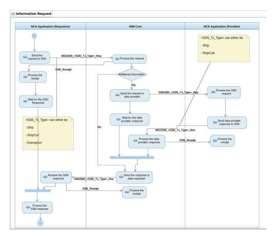
The process flow illustrates the case where the *data provider* can talk XML with SafeSeaNet.
