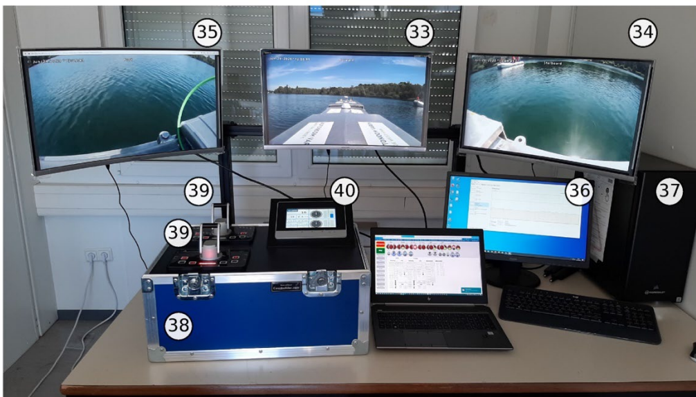
Figure 15: I-SCC realised in H2H for remote control of the Cogge, copied from Peeters et al. (2020).
