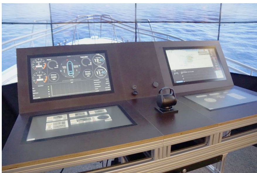
Figure 31: Prototype of a mobile ship bridge for a ROC, copied from Lamm (2022).
