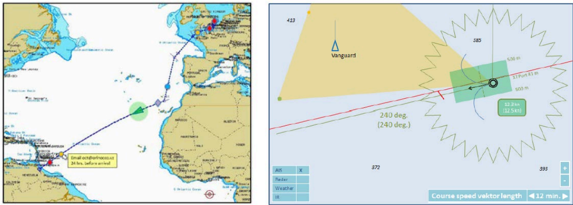
Figure 10: ECDIS-like display for spatial overview (left) and zoom in (right) on egocentric information on a specific ship, copied from Porathe (2014).
