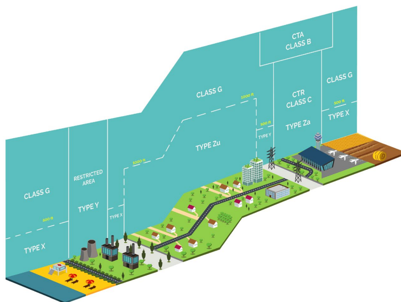
Figure 62: Airspace volumes for drones in Very Low Level airspace, copied from CORUS Consortium (2019a).
