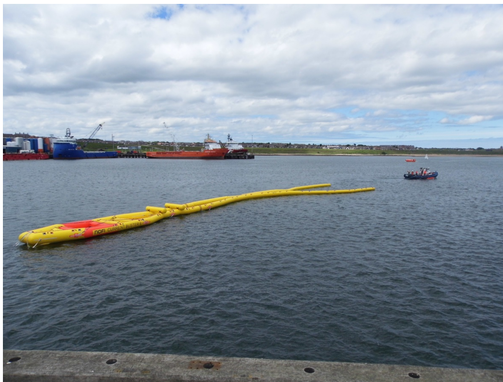
Figure 2 EAS North Sea (Aberdeen). Training for the MS equipment operators. Deployment of the Current Buster.
