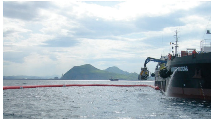
Skimmer and boom deployment, oil spill exercise with EMSA oil-spill response vessel Monte Arucas
