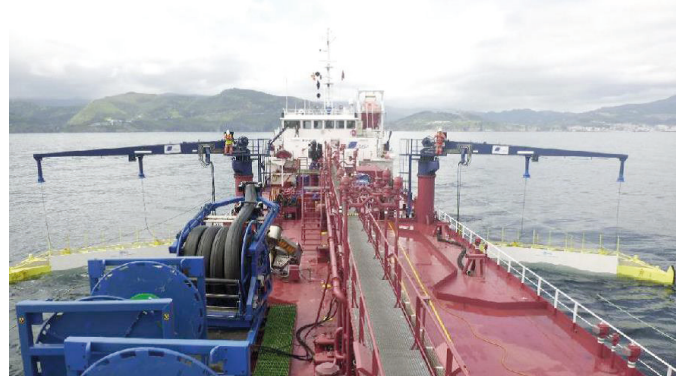
Deployment of the boom in U-configuration, oil spill exercise with EMSA oil-spill response vessel Monte Arucas
