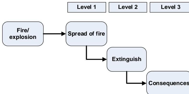
**Fig. 8.39: High-level event sequence for fire/explosion on cruise ships (based on SAFEDOR FSA on Cruise)**
