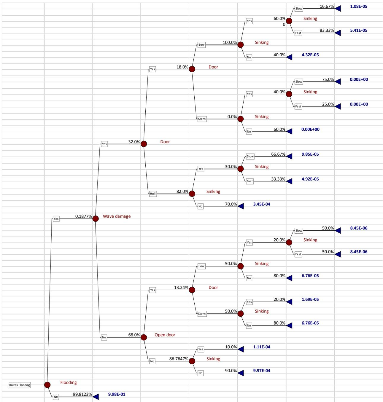
Fig. 8.53: Flooding risk model RoPax from SAFEDOR FSA on RoPax
