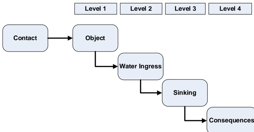
**Fig. 8.41: High-level event sequence for contact of cruise ships (based on SAFEDOR FSA on Cruise)**
