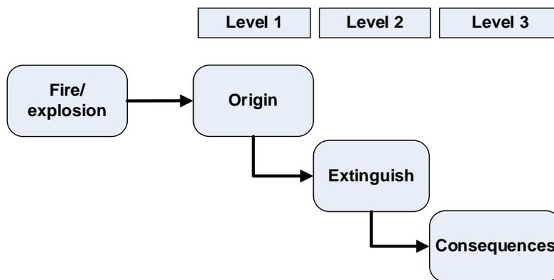
**Fig. 8.40: High-level event sequence for fire/explosion on RoPax ships (based on SAFEDOR FSA on RoPax)**
