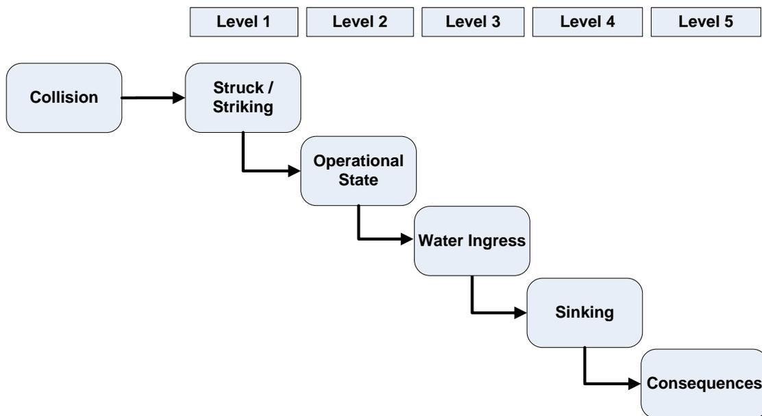
Fig. 8.37: High-level event sequence for collision of Cruise and RoPax (based on GOALDS)
