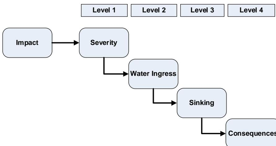
**Fig. 8.42: High-level event sequence for contact/impact of RoPax ships (based on SAFEDOR FSA on RoPax)**
