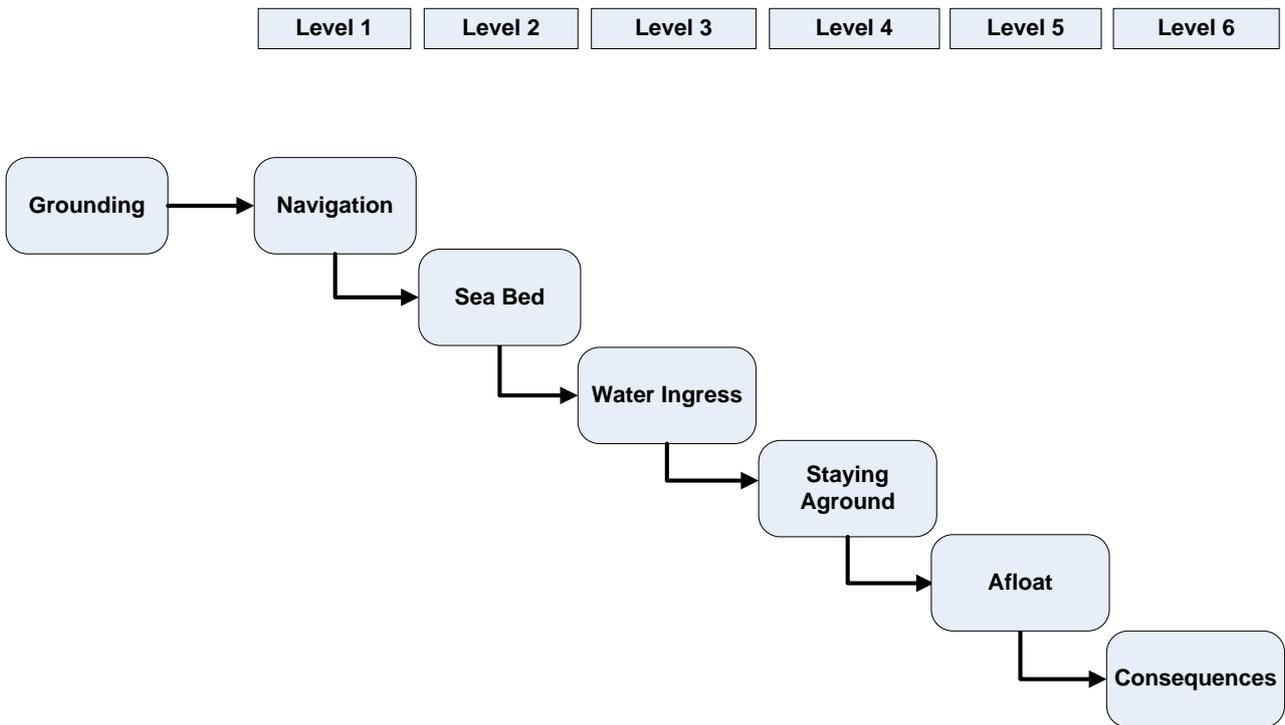
**Fig. 8.38: High-level event sequence for grounding of Cruise and RoPax (based on GOALDS)**
