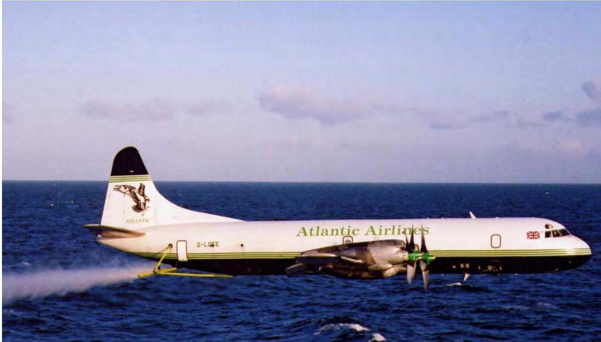
Figure 14. Lockheed Electra aircraft spraying dispersant
