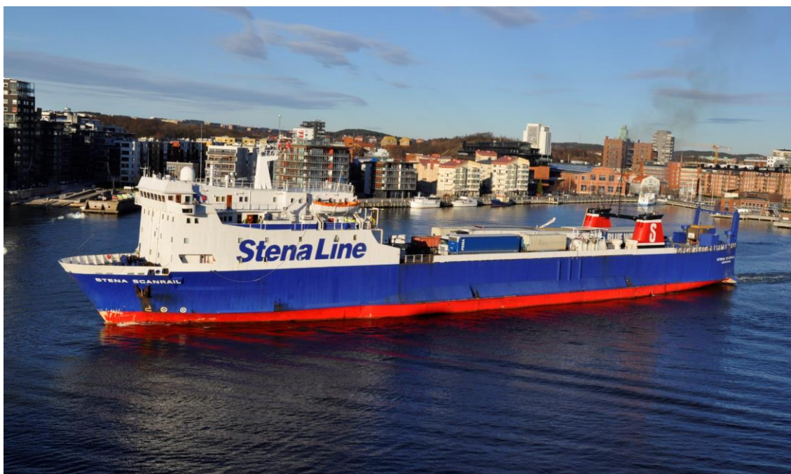
Figure 2: The Stena Scanrail with methanol tank installation forward of the port side funnel (Photo by Joanne Ellis, courtesy SPIRETH Project)
