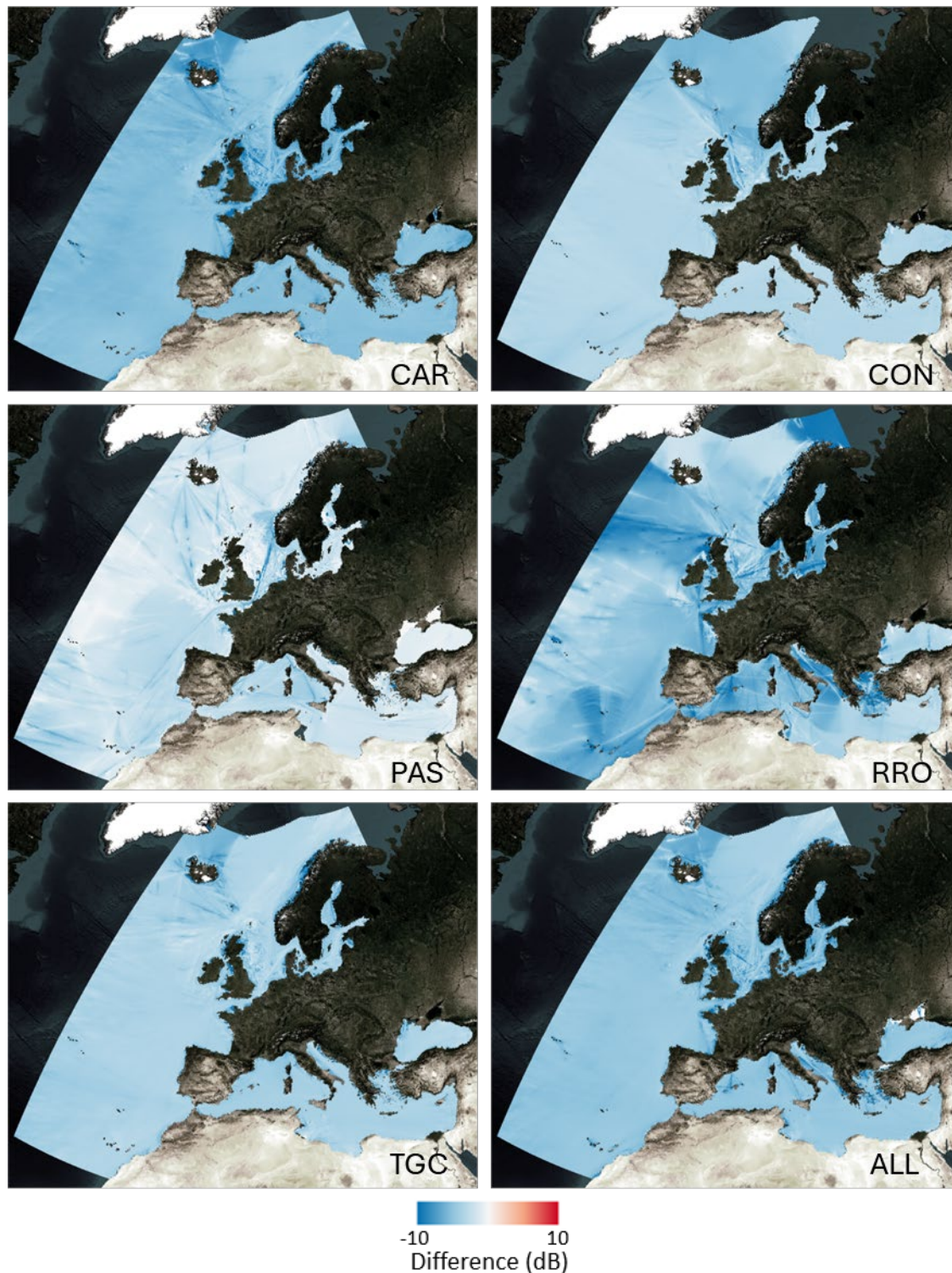
Figure 57 Difference in forecast sound pressure level (SPL; dB) for different vessel categories between BAU and URN scenarios. The sound map layers are annually averaged for 2050 at 63 Hz.
