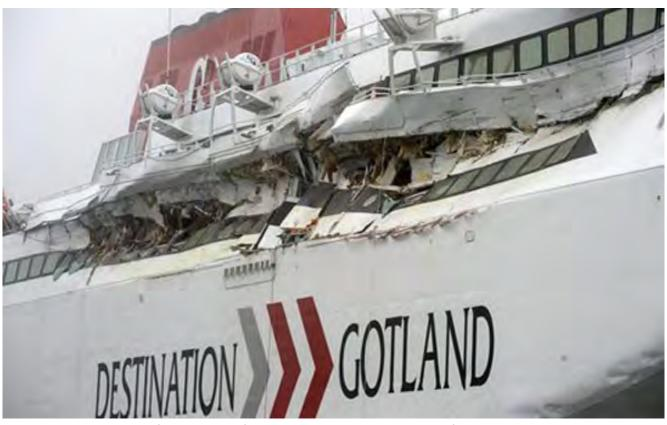
Substantial damage to the ferry Gotlandia II, after the collision with the Gotland at the port of Nynashamn (Sweden) during July 2009.
