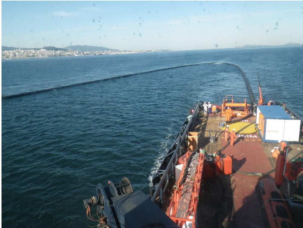
Figure 2 Weir boom deployed from the Ria de Vigo during sea trials
