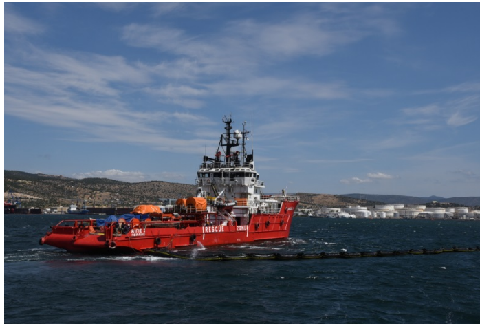
Fig.6. Aegis I towing the boom in J formation
