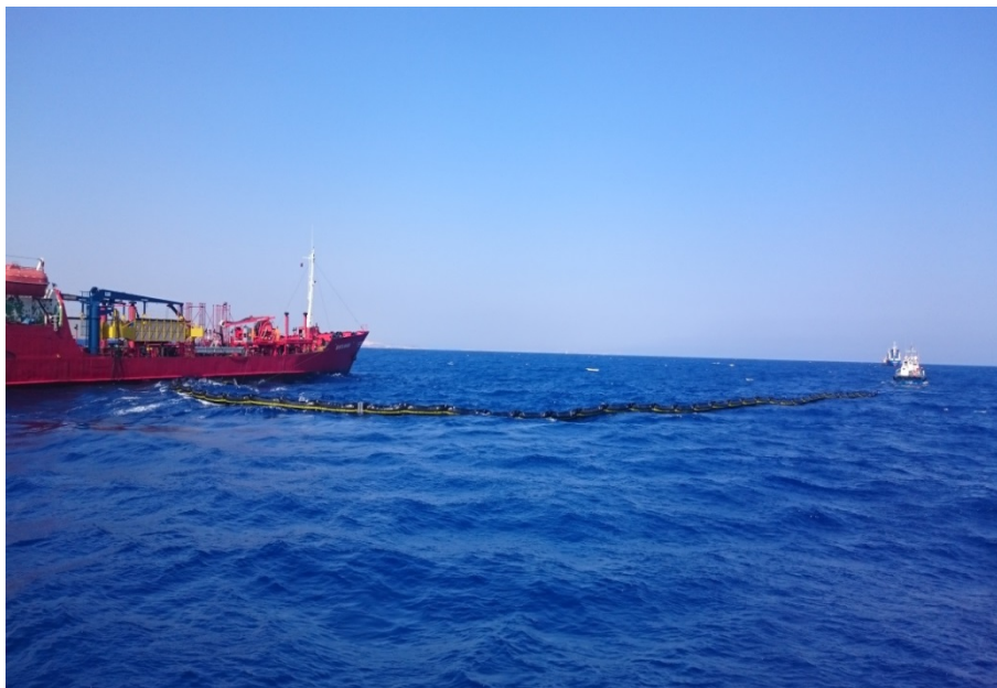
Fig.10. Santa Maria (EMSA) – Desmi Ro-boom 2000 in “J” formation
