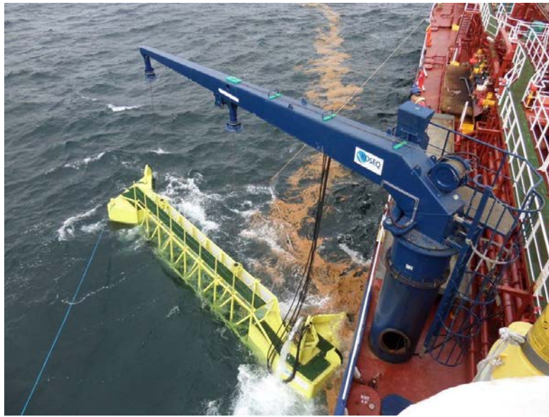
Fig.5. Forth Fisher recovering the oil simulant
