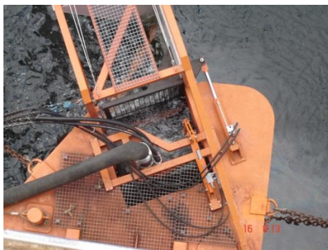
Pictures 8 Hydraulic connections to Sweeping Arm
