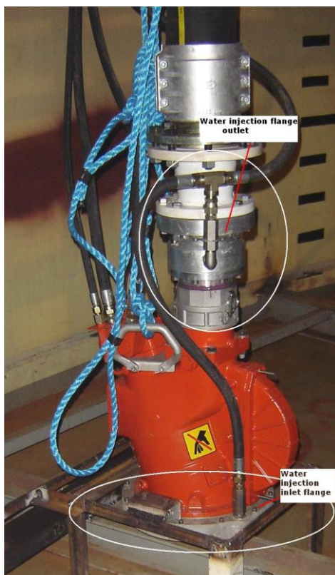
Picture 6 Water Injection Flanges DOP
